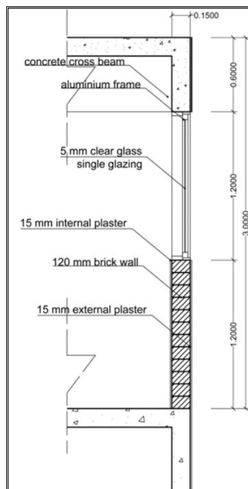
Figure 2. Floor to ceiling structural and wall detail
