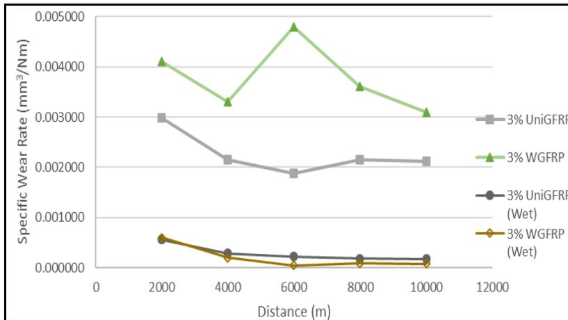
Figure 2. Specific Wear Rate of 3 wt. % Nano-modified Unidirectional and Woven GFRP Composite under dry and wet environment
