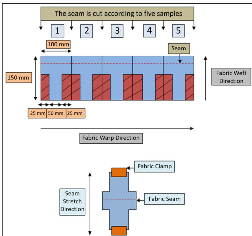
Figure 2. Preparation of sample for seam strength test
