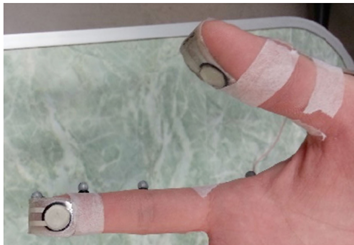
Figure 3. Flexi-force sensor position
