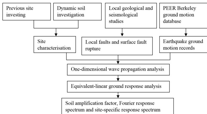
Figure 1. Steps in site-specific ground response analysis
