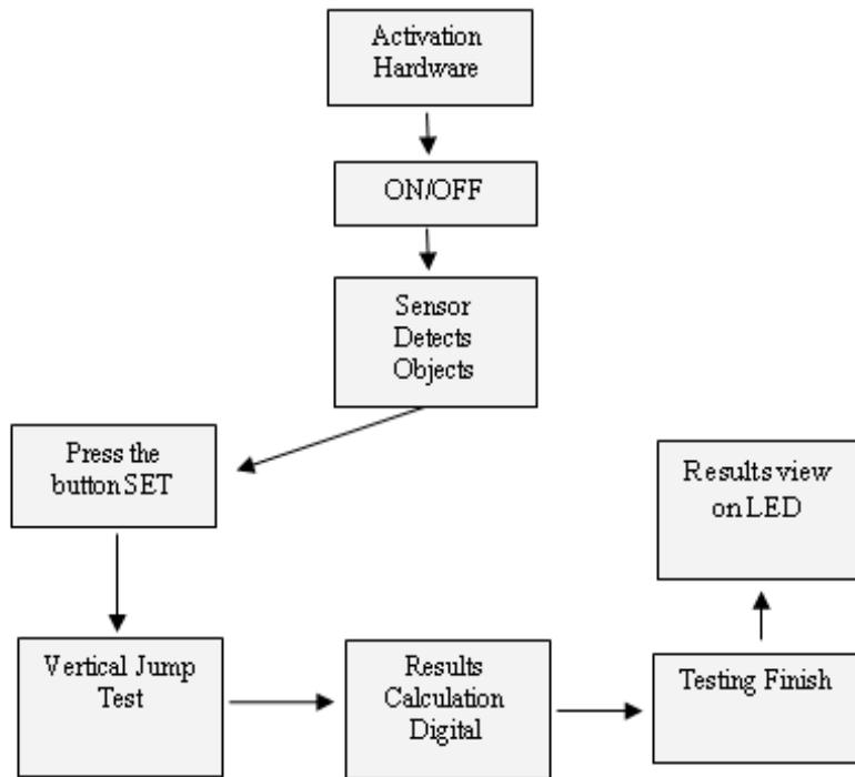
Figure 7. Structure of the workings device system
